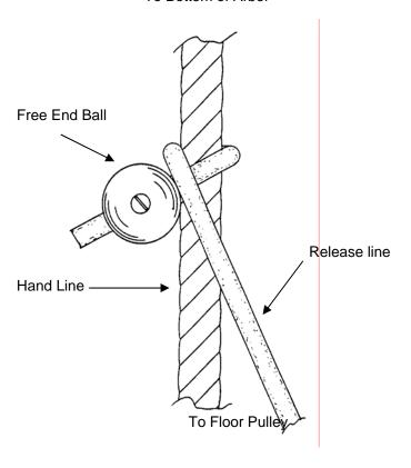
This type of system requires some practice and angle at which the release line is attached to the handline is critical. Too little of an angle, and the curtain will not deploy. Too much of angle and the release line won't hold. Additional weight may be added to the release line either before of after the floor block to aid in the quick freeing of the line. If you are having difficulty with setting your release, contact a professional stage rigging company.
